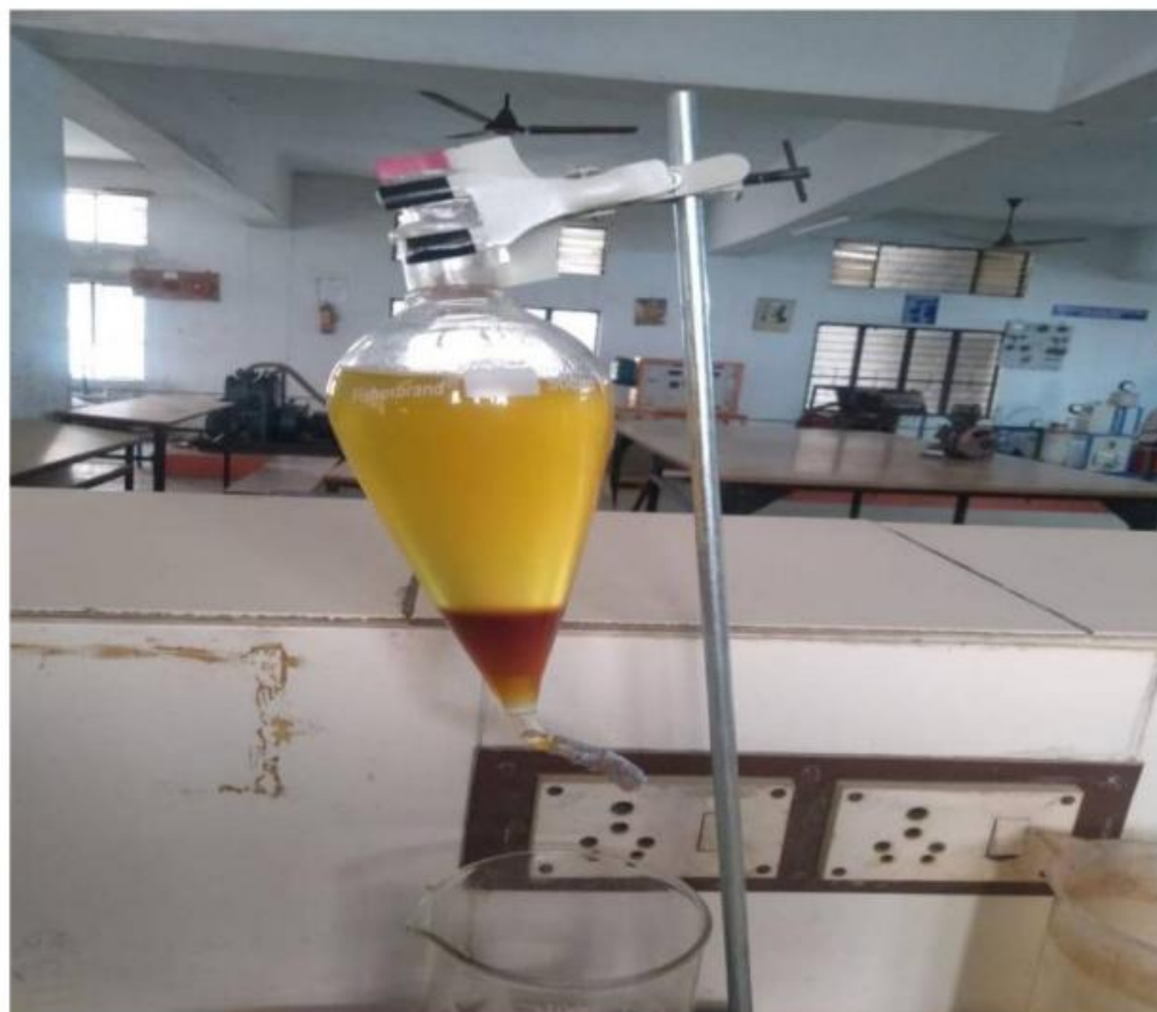
Fig: 3.2 Separation of Glycerol and Esters
