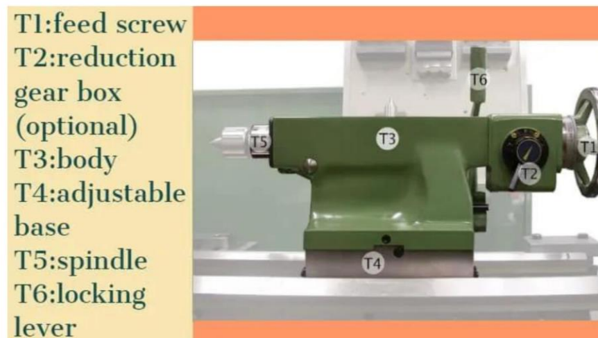
Figure 1. 6: Tail Stock of a Lathe Machine & Their Parts
