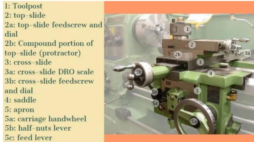
Figure 1. 7: Carriage of a Lathe Machine & Their Parts
