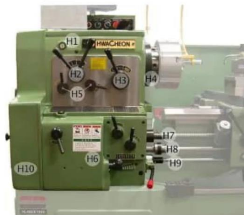
Figure 1. 5: Head Stock of a Lathe Machine & Their Parts
