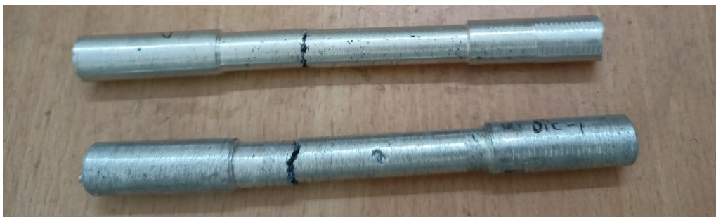
Fig 4.9 Tensile Test Specimen after testing
