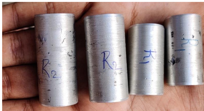
Fig 4.11 Compression Pieces after Machining
