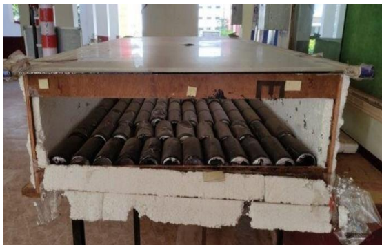
Fig: 3.5 flat plate collector
