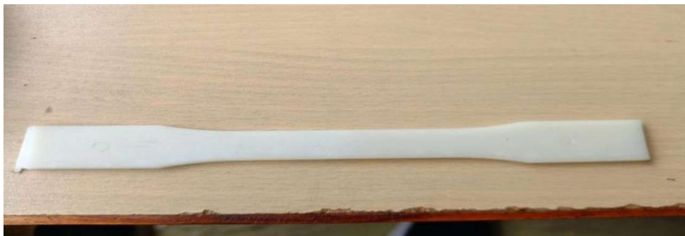
Fig 4.2 :- sample tensile test specimen after injection moulding
