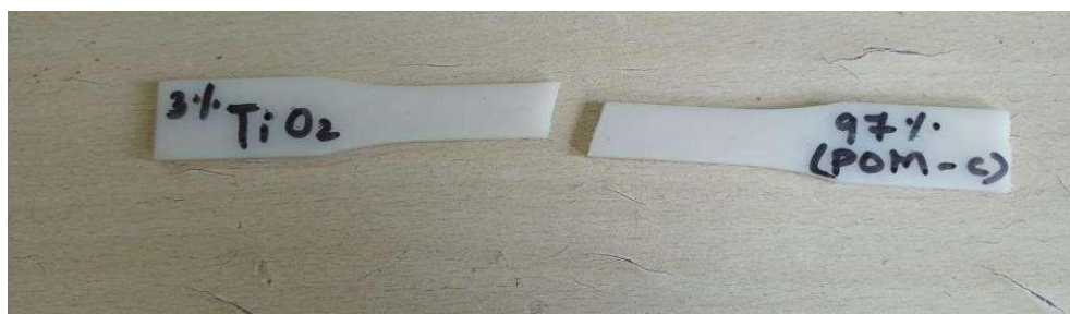
Fig 4.6 : Specimen after the test (97% wt POM-C, 3% wt TiO 2 )
