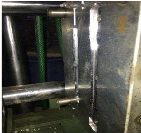
FIGURE 3.1:- Tensile and Flexural specimens' mould fastened to machine for producing the tensile and flexural specimens ( mould with ejector pins in original position )
