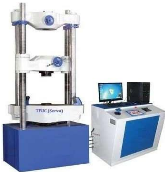
Fig 4.1:-Universal testing machine(UTM) for performing tensile test on the specimen
