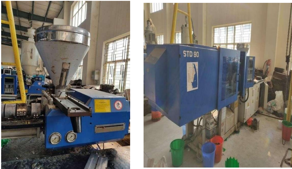
Figure 2.4: Twin Screw Extruder fitted with circular die powered by servo motors operated at 175°C with a rotor speed of 100 rpm for 5 minutes.
