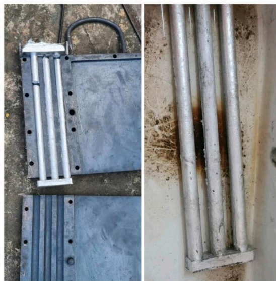
Fig 3.8 Casted aluminium bars
