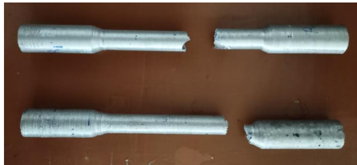
Fig 4.9 Tensile Test Specimen after testing (ASTM-E08Standard)
