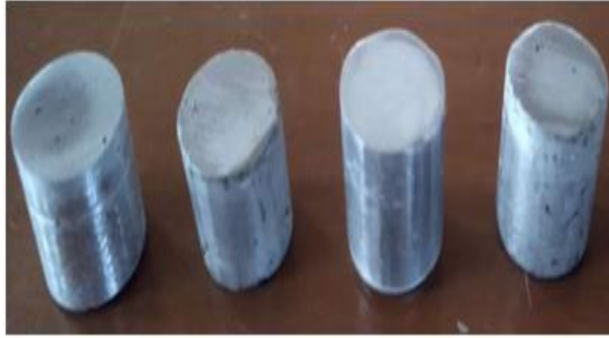
Fig 4.15 Hardness test Specimens after testing
