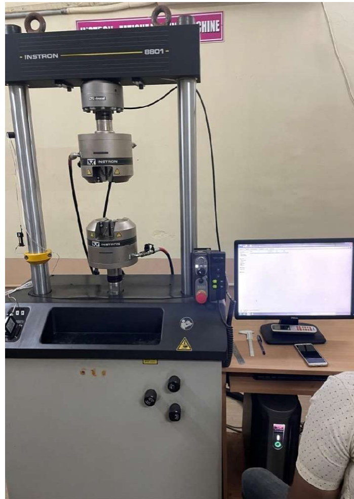
Fig 4.2 Universal testing machine
