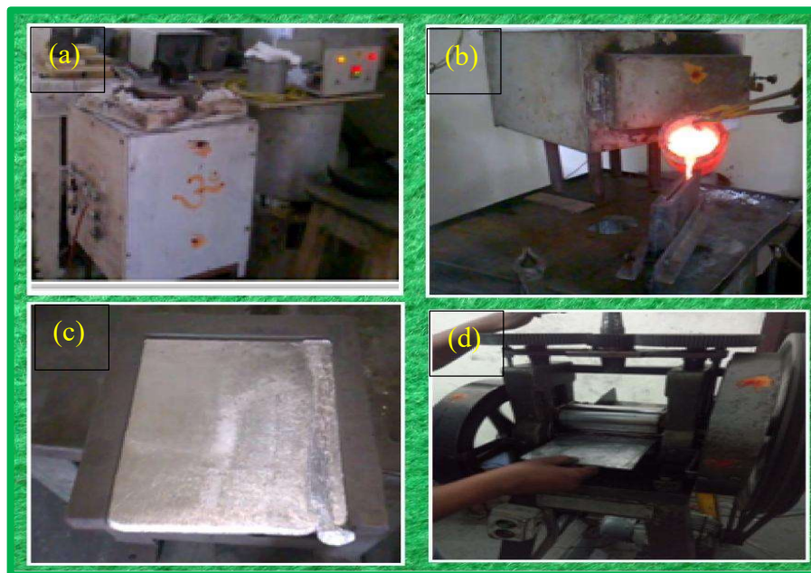
Fig 3.1 Fabrication process of Al-Mg-Mn alloy
