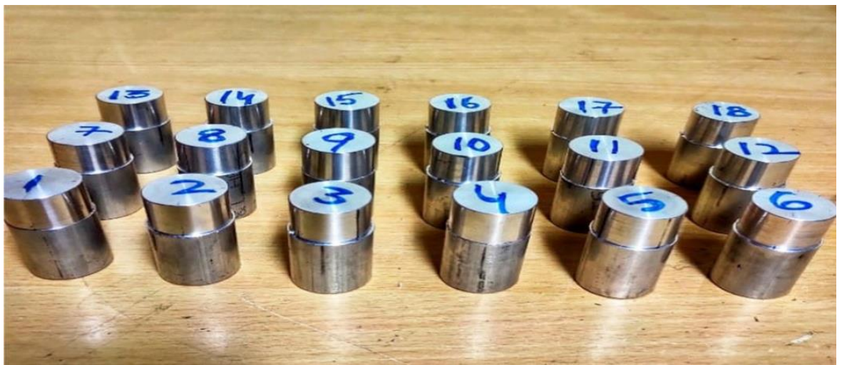
Figure 4.1. AA6061-T6 Cylindrical Work Pieces after Machining
