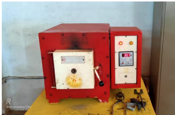
Fig: 4.6 Muffle Furnace
