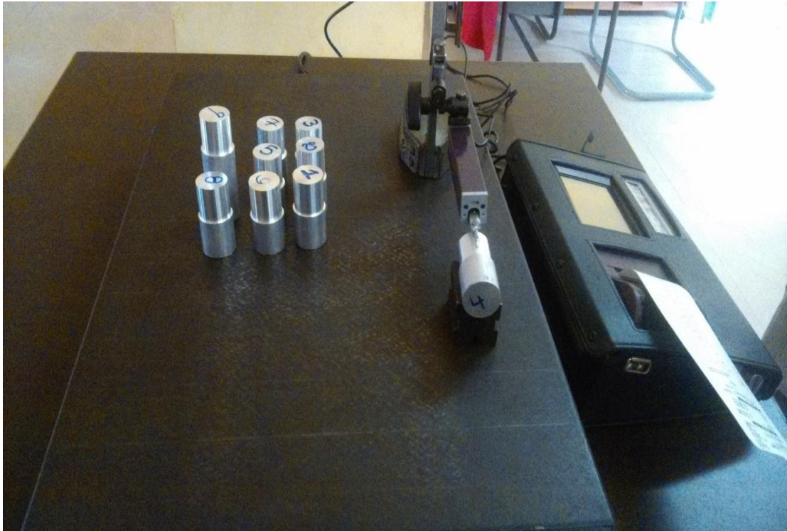
Figure 4.6. Surface Roughness Measurement Set-up
