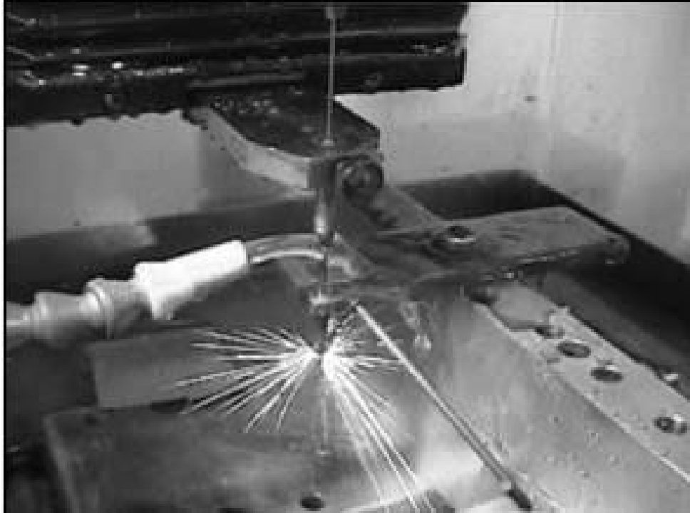
Figure 1.3 Generation of Spark in WEDM
