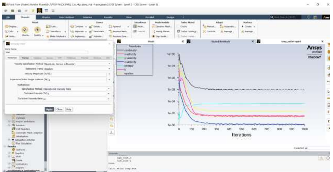
Fig 5.2.2 Scaled residuals for the radiator at 2m/s
