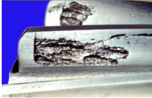
Fig.1.11: Macro pitting on Gear Teeth
