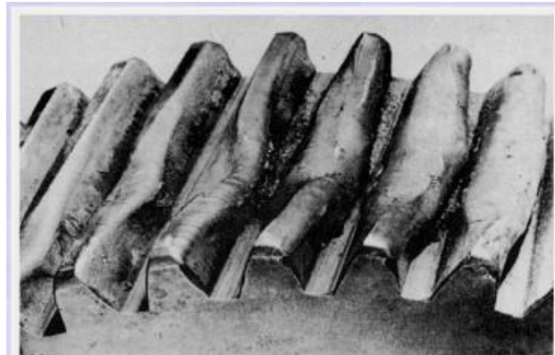
Fig.1.12: Damage to a case-hardened gear resulting from overheating associated with insufficient lubrication
