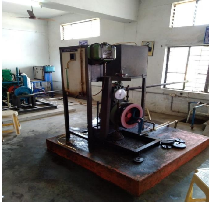
Fig 4.2: Four Stroke, Single Cylinder, Vertical Diesel Engine
