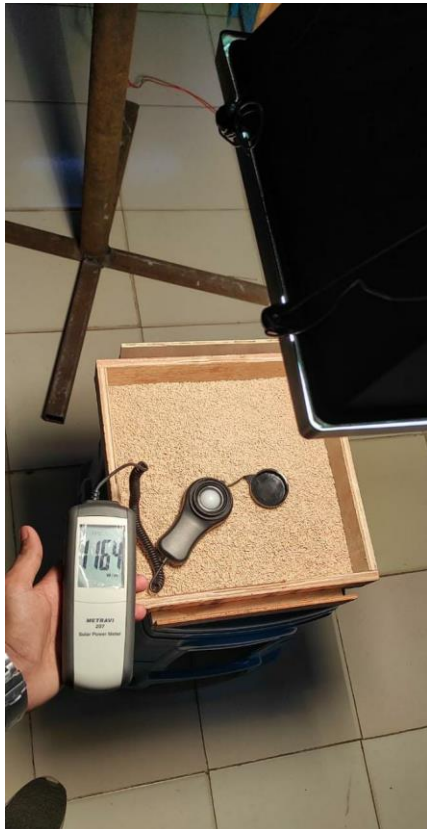
Fig 4.10 solar power meter
