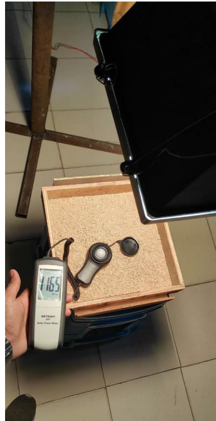
Fig 4.11 solar power meter (readings)
