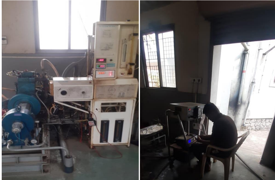
Fig 3.1. Single cylinder, CRDI with EGR, open ECU and Emission Analyzer
