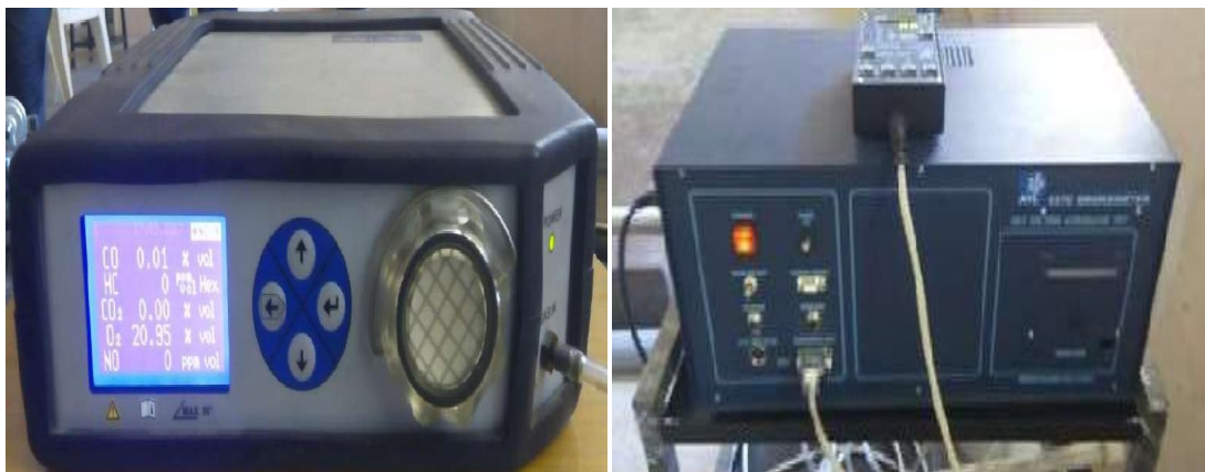
Fig 3.3. Photographic view of the emission analyzer
