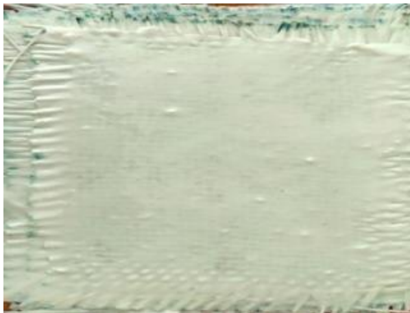
Fig 3.3 Solidified composite sheets after curing 48 hours at room temperature
