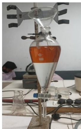
(e) Final stage of water washing
