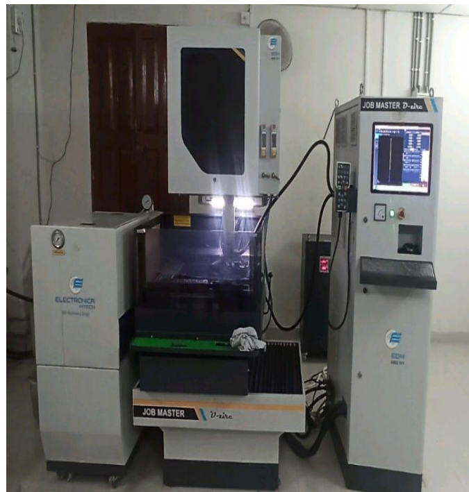
Figure 4. 1 : WEDM Experimental Setup
