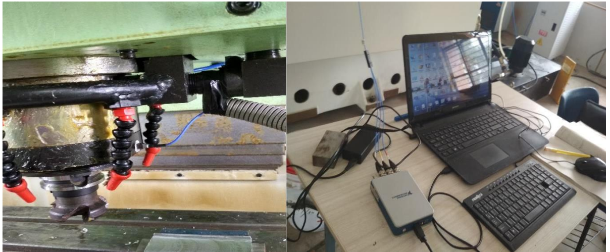
Fig 3.7.1 : Sensor and systematic arrangement for force analysis
