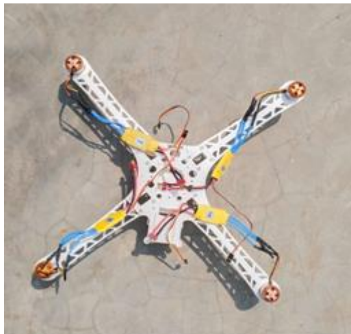
Figure 3.24 Attaching esc and motors' to frame
