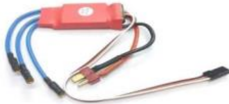
Figure 1.8 Electronic Speed Controller
