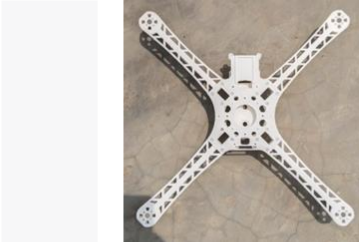
Figure 3.23 initial frame set up
