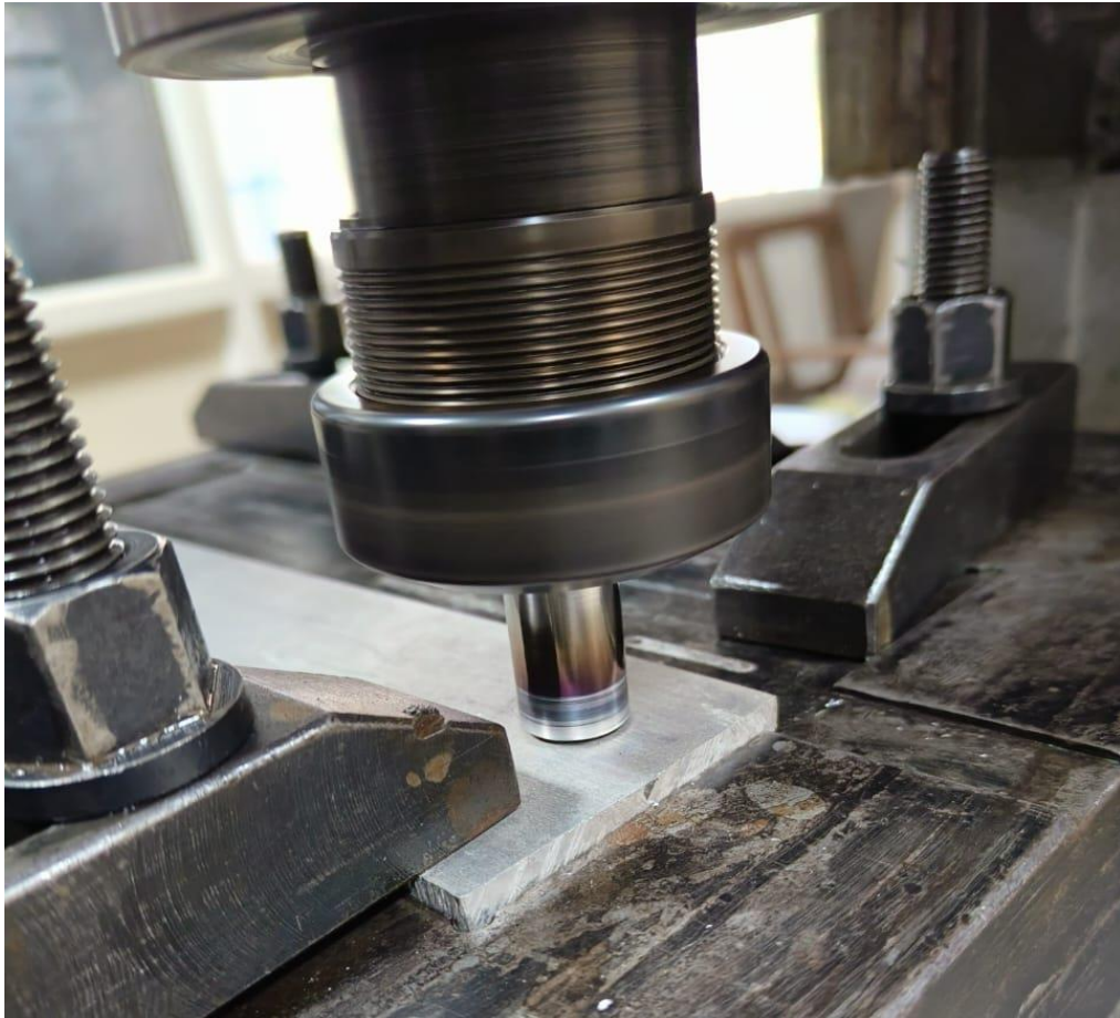
Figure 1.6 Friction stir welding on similar Aluminium alloys
