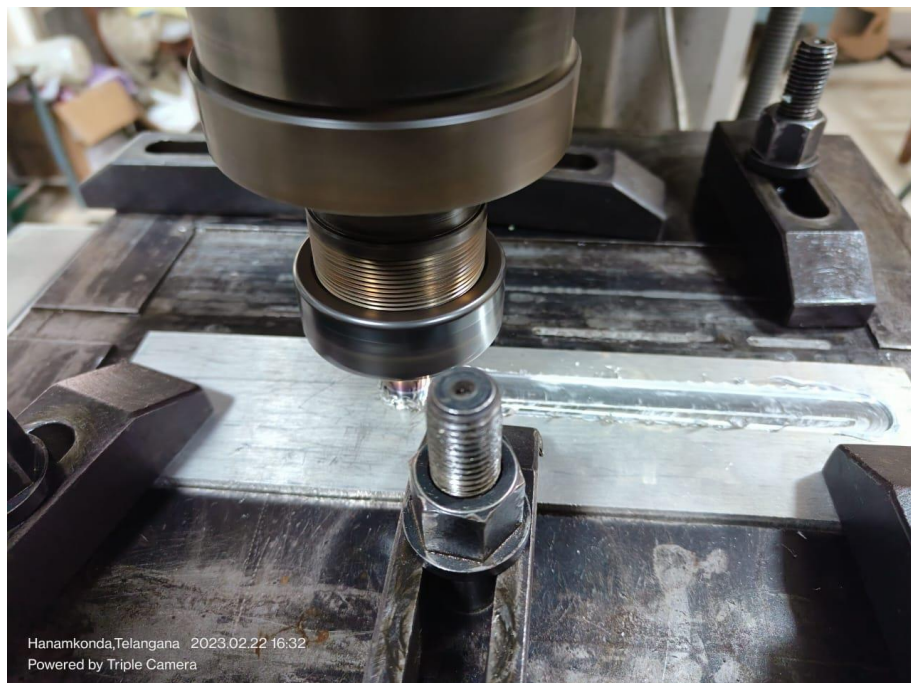
Figure 3.4 FSW process on dissimilar Aluminium alloys
