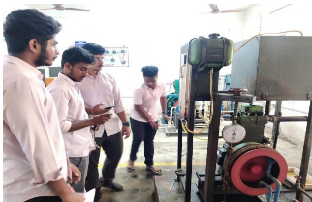
Fig 4.3 four-stroke single cylinder diesel engine
