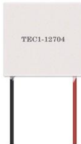
Fig 5.1 Thermoelectric Peltier Module
