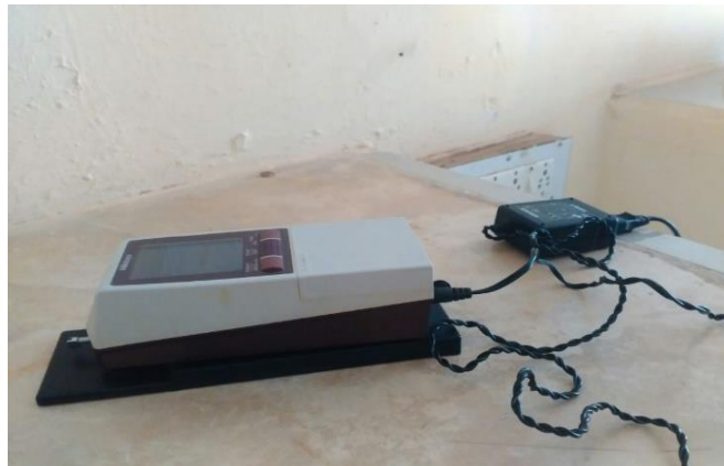
Fig 4.7 Surface Roughness Tester measure
