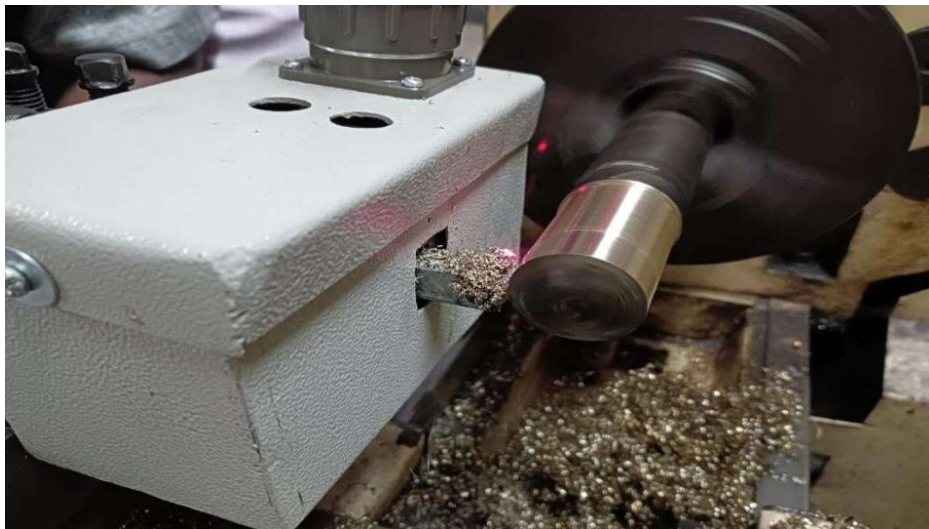
Figure 4.2 Workpiece under turning operation
