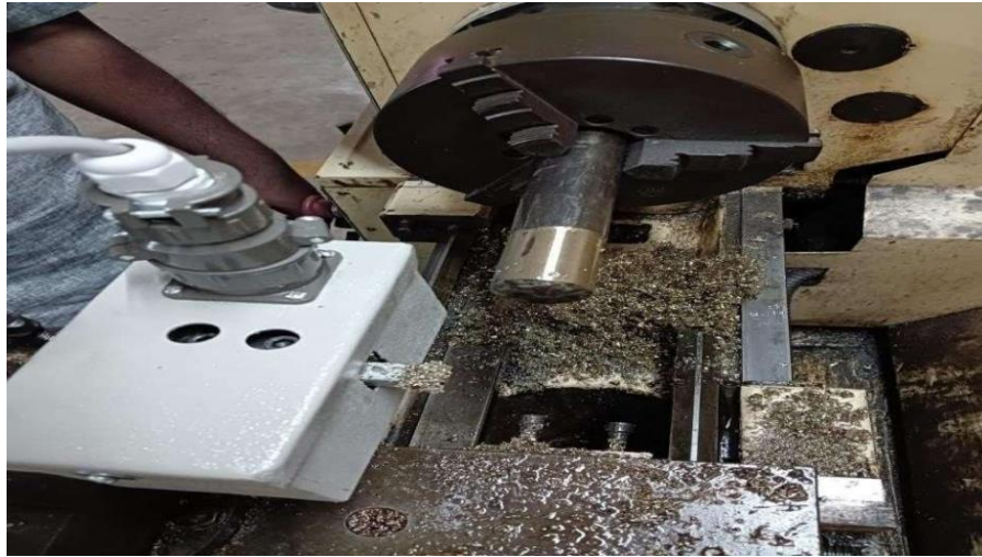
Figure 4.1 Clamping of the work piece
