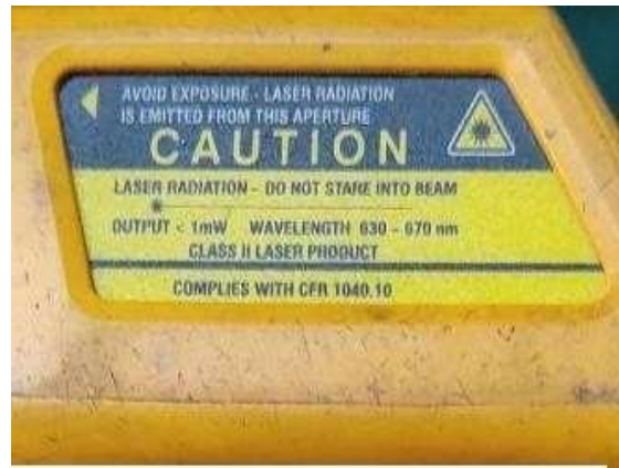
Figure 1.9(b) Cautions when usage of temperature gun
