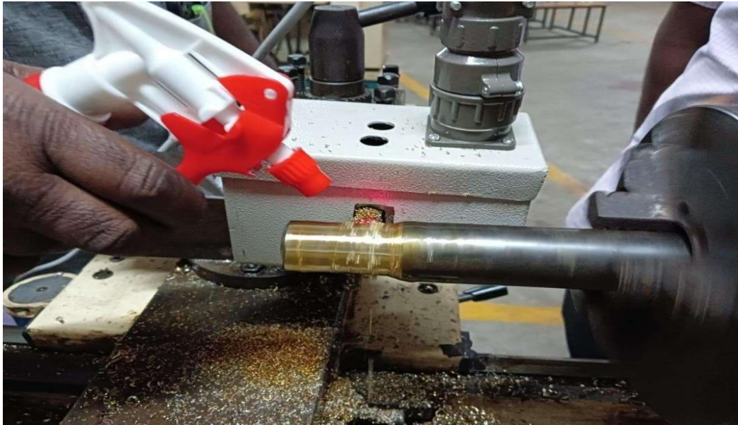
Figure 4.3 Apply cutting fluids during machining process
