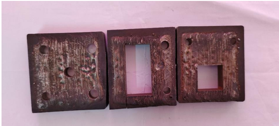
Figure 5.2. TIG Cladding Samples
